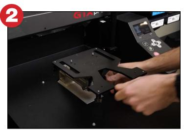
**Step 2:**Adjust the height of the platen and tighten the locking lever.
