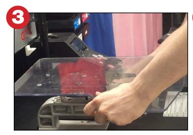
**Step 3:** Insert the T-Lock Shoulder Insert into the T-Lock Base. The insert is reversible, so ensure it's flipped to the correct side for what you want to print.
